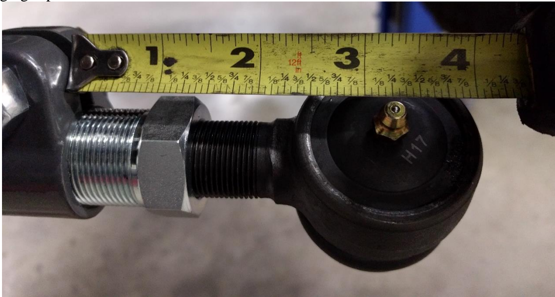
Figure 4. Tie Rod End Adjusted 3.25" Out, 1/4" From Maximum
